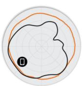
Figure 4. R610 2.4GHz Elevation Antenna Patterns
