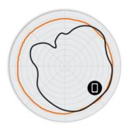
Figure 3. R610 5GHz Azimuth Antenna Patterns
