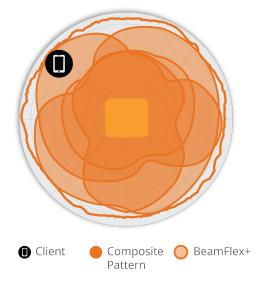
Figure 2. R610 2.4GHz Azimuth Antenna Patterns
