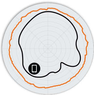
Figure 2. E510 2.4GHz Azimuth Antenna Patterns
