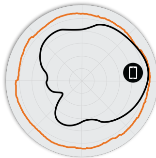
Figure 3. E510 5GHz Azimuth Antenna Patterns
