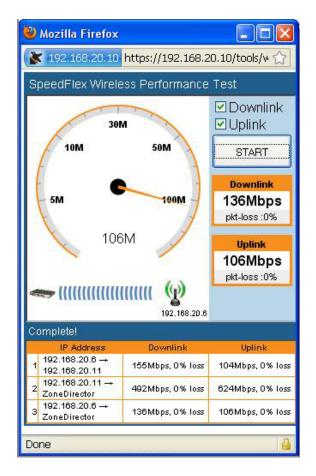
Figure 3. SpeedFlex<sup>™</sup> is a unique wireless performance test tool integrated within the Ruckus family of centralized controllers that measures the Wi-Fi throughput of associated wireless LAN clients.
